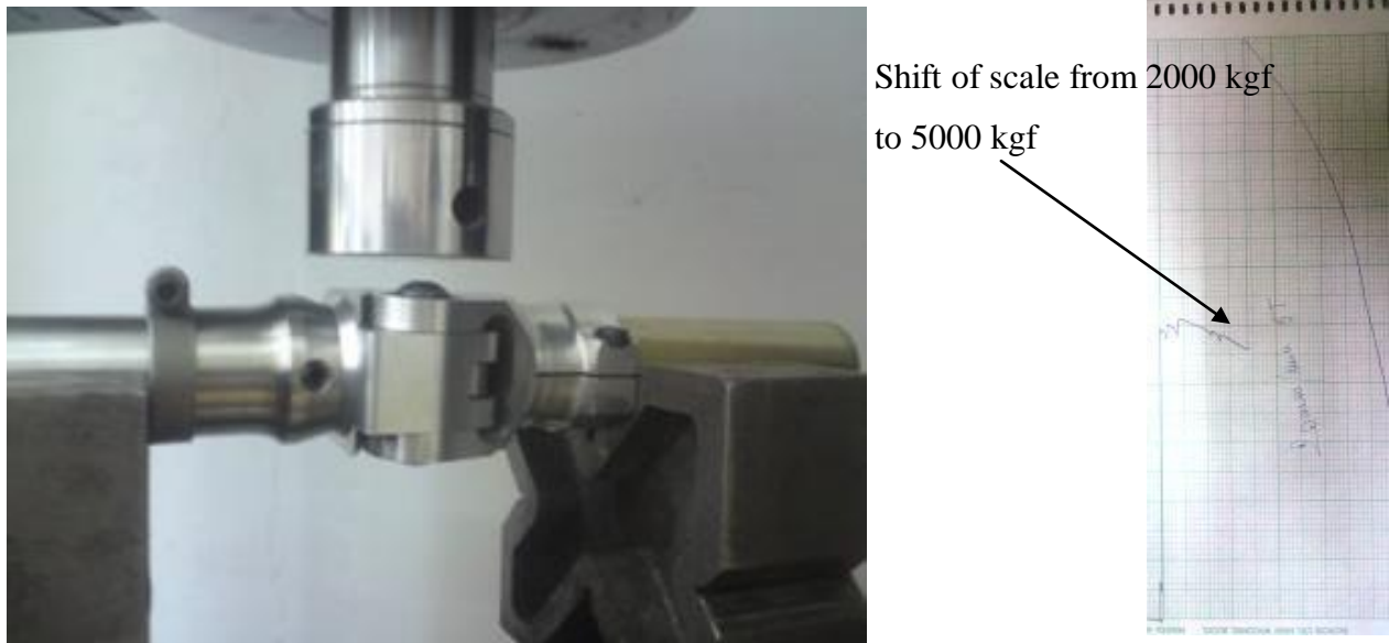
Figure 4. a. The second setup, b. Force-strain plot of the second configuration.
