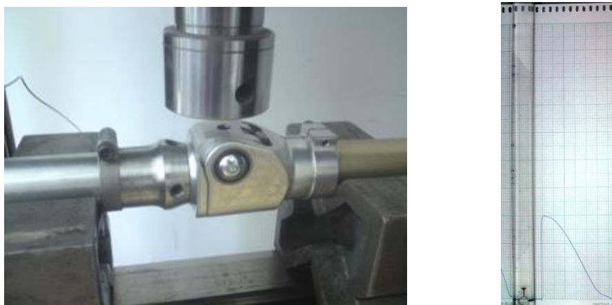
Figure 5. a. The third configuration, b. Force-strain plot of the third configuration. The vertical scale represents 2000 kgf.
